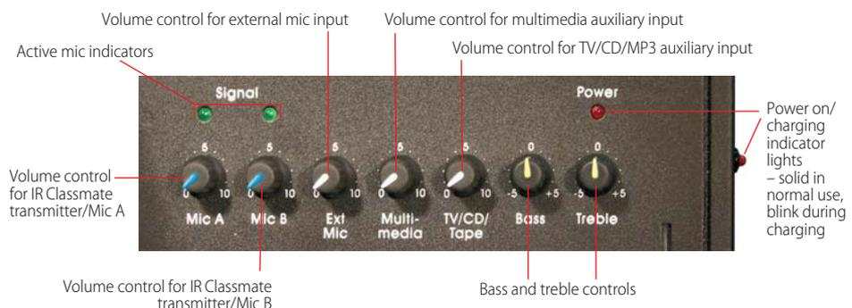
**IR Classmate and IR Classmate +** The IR Classmate+ has all the features of the IR Classmate with the addition of a remote volume adjust feature for use with a Swift TX transmitter.
