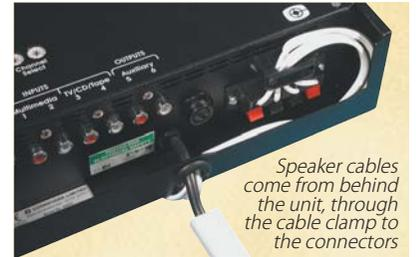
Speaker cables come from behind the unit, through the cable clamp to the connectors
