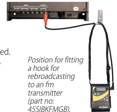
Position for fitting a hook for rebroadcasting to an fm transmitter (part no: 45SIBKFMGB).
