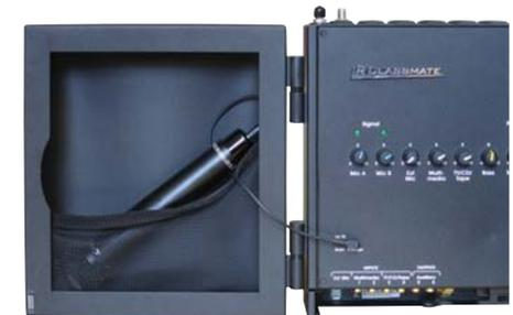
Handheld transmitters are charged with a 2.1mm plugged charge lead (part no. X0IR00)
