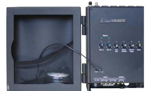
Swift tx transmitters are charged with a 1.3mm plugged charge lead (part no. X0DIV00)
