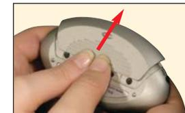
The battery door is treated with a clear anti-slip finish to reduce the tendency to move when worn.
