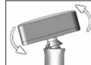
**DO NOT** pull the sound processor straight out or **you may damage your sound processor.**
