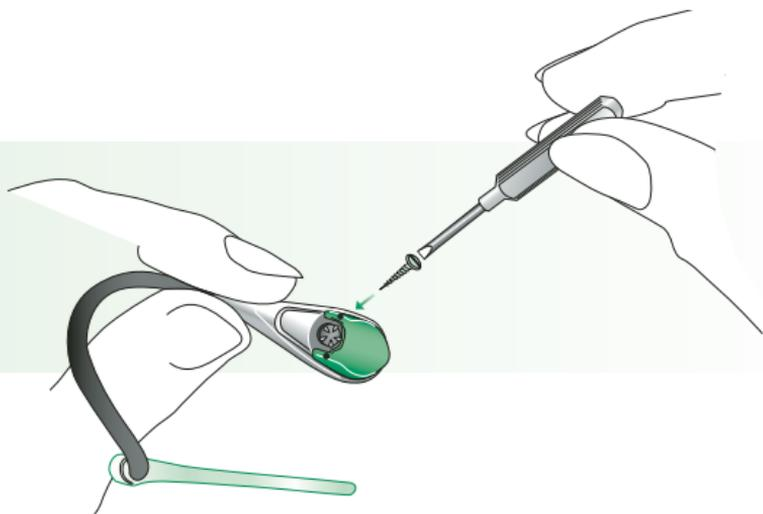
**⚠** The screws must be removed each time the battery is replaced!
