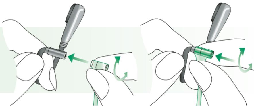
**⚠** Never wear EduLink S without a retention lock, and be sure not to poke the retention lock down the ear canal!
