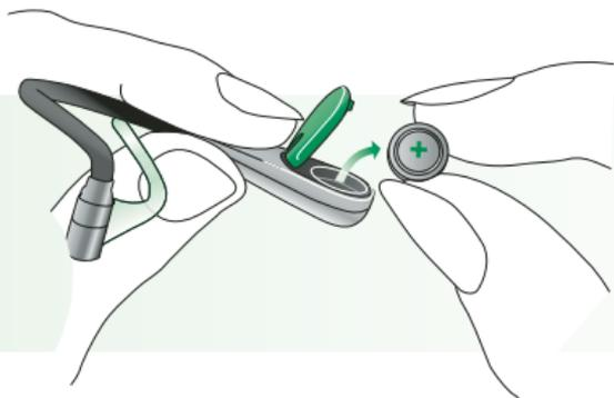
b) Lift up the battery compartment cover at a right angle and pull it away in the direction of the battery compartment.
