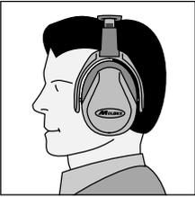
When putting on the ear muff, the headband needs to be positioned in the middle of the head and the cushions need to cover the ears.
