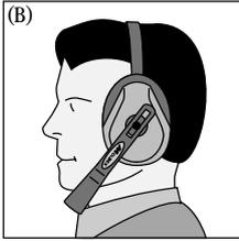
(B) M2 under chin: When putting on the ear muff with the headband under chin, the black/flexible strap needs to be inserted in the loop on the top of the cups (see: a + b) and position the strap in the middle of the head. The cushions need to cover the ear.
