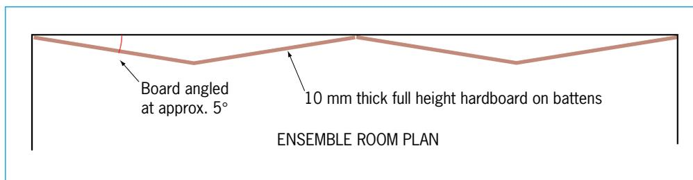
**Figure 7.5.4:** Simple acoustically diffusing elements
