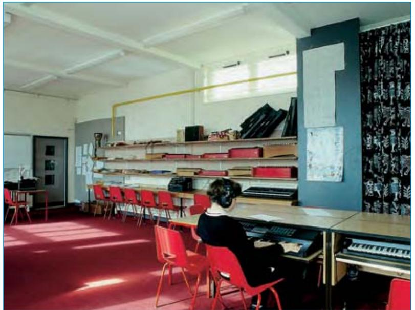
were hard, resulting in an unacceptably long reverberation time of 2 seconds. Standing waves and flutter echoes were likely due to parallel walls and hard surfaces.
