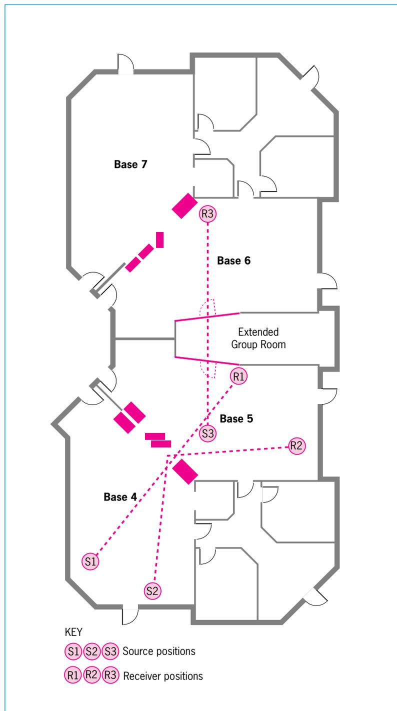
By comparing the two figures, it is evident that the reduction in sound level with distance between bases 4 and 5 is very modest compared with the large reduction between bases 5 and 6 (ie across the partition). This is clearly reflected by the subjective impressions of teachers who are disturbed by noise from an adjacent classbase on the same side of the partition but are not disturbed by classbases beyond the partition.
