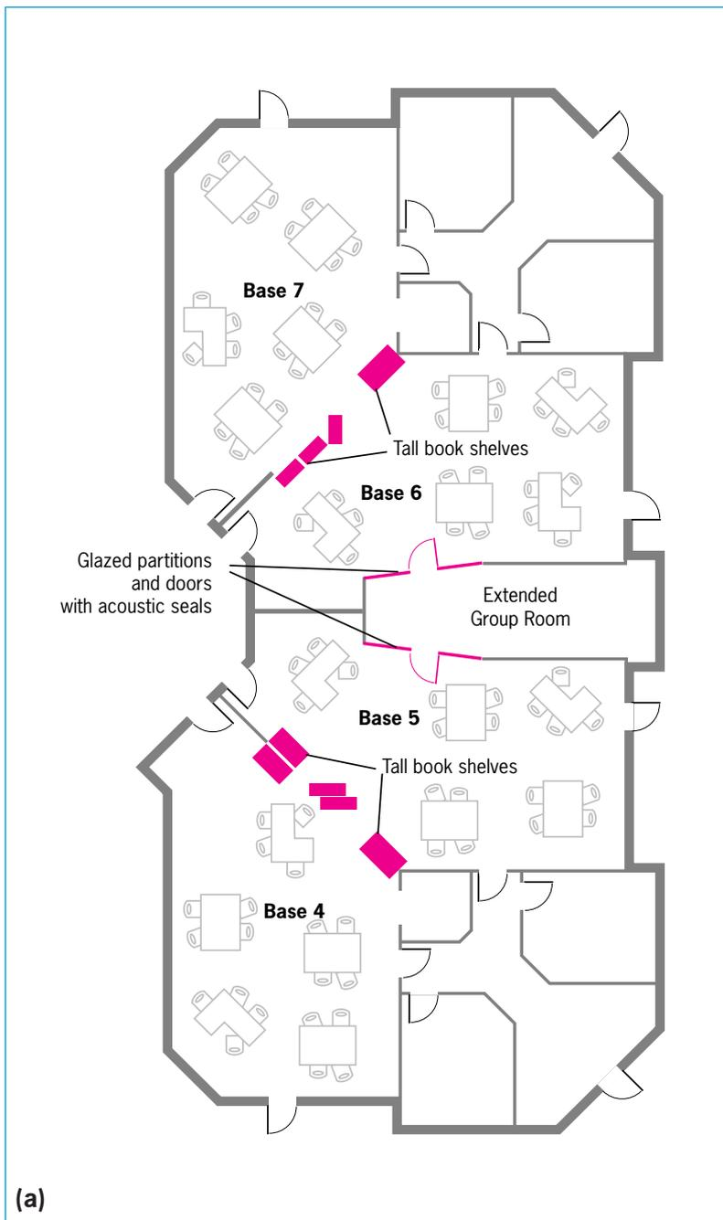
**Figure 7.3.2:** Arrangement of open-plan teaching spaces following modifications
