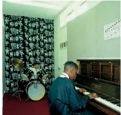
that curtains can be very effective in reducing mid-frequency reverberation time. Because of the number of variables combining to affect the reverberation time in a room including volume, the weight and location of curtains, surface finishes and furniture, the results shown here are indicative only. The graph shows that the ensemble room at 13 m<sup>2</sup> has a measured RT of 0.7 to 0.8 seconds, within the range given in Table 1.5 of 0.6 to 1.2 seconds for an ensemble room.
