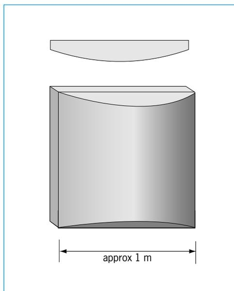
**Figure 7.1.4:** Example of acoustically diffusing panel
