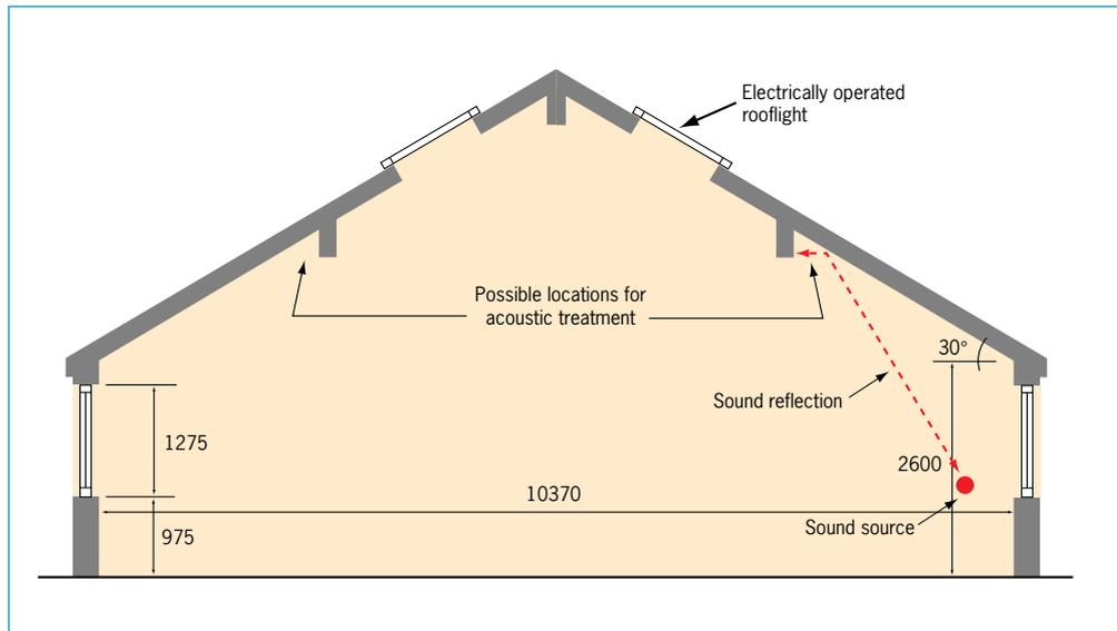
the sound field. For effective diffusion, projections of 0.3 m to 0.5 m are necessary. However, such projections should be distributed over the whole ceiling area; a single large projection can lead to a prominent and potentially disturbing reflection, as in this case.
