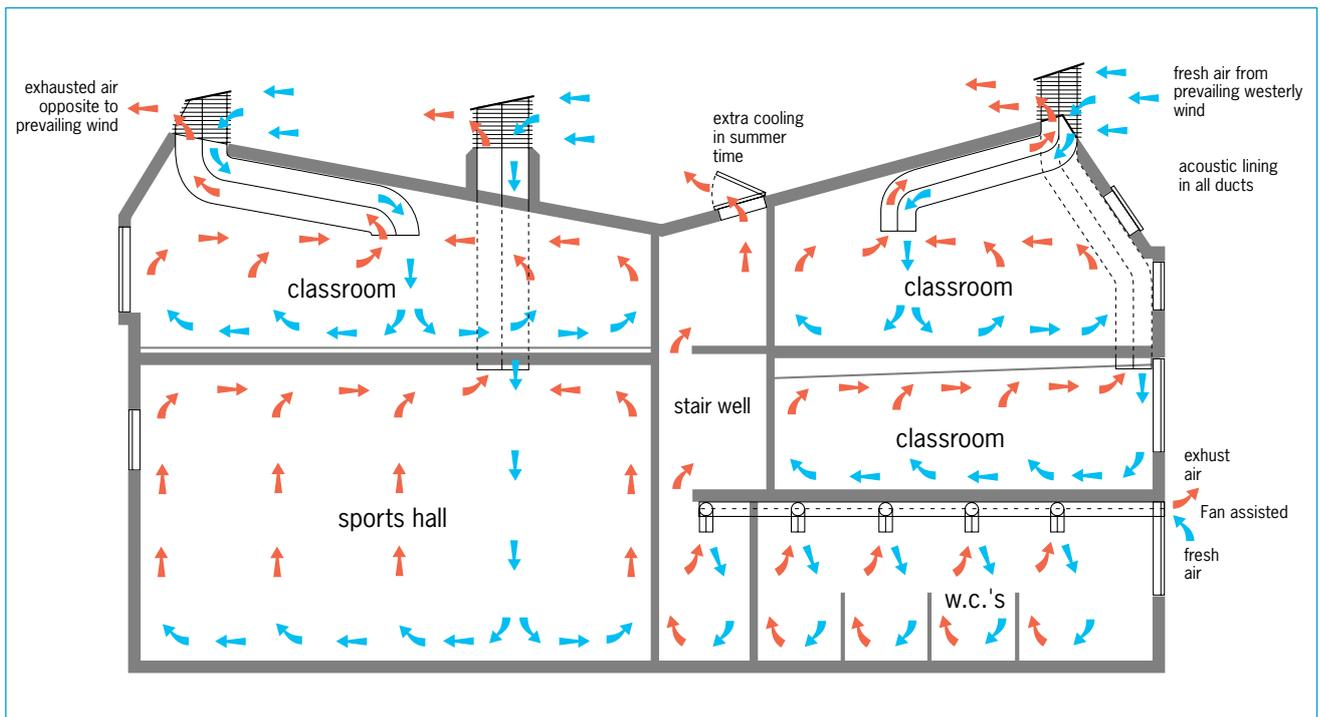
carried out with the ventilation system open and closed. The results did not display any significant change in level nor was there any significant variation in the sound pressure level around the room.
