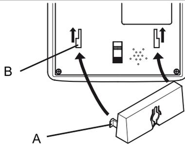
5. Position the phone so that the screws on the wall fit into the slots in the bracket, then slide the phone downwards until it is hanging on the screws.
