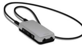
**RONDO:** For the best orientation of the integrated T-Coil, please wear the RONDO with microphone on top position.
