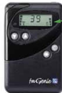
**1** Before you switch off the fmGenie unit for the last time of the day check the battery display.
