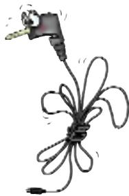
Don't remove shoes by pulling on the leads – unclip the shoe itself.
