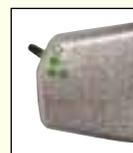
Select 'FM' (●) to reduce the pickup of ambient noise from around the hearing aid by 20dB.
