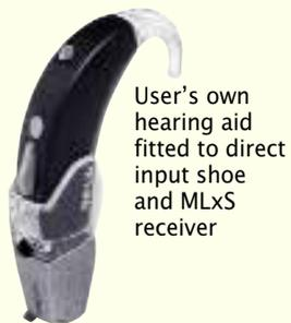
User's own hearing aid fitted to direct input shoe and MLxS receiver
