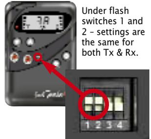
Under flash switches 1 and 2 - settings are the same for both Tx & Rx.
