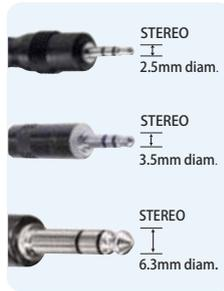
As well as coming in different sizes, jack plugs are available with different numbers of electrical connections – it's not complicated, simply look for the number of black bands on the plug... one for mono, two for stereo.
